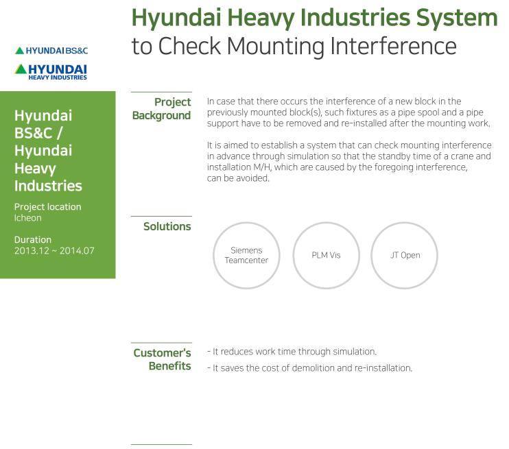
**Highlights** - Developing mounting interference check system and a JT converter for mounting work.
